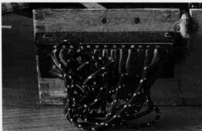
Figure 9. Detail of plugboard attached to left side of A16992.
