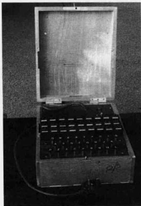
Figure 10. Digital counting device mounted in the case of M16264.
