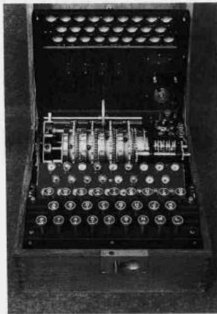
Figure 3. G-312 with inner lid open.
